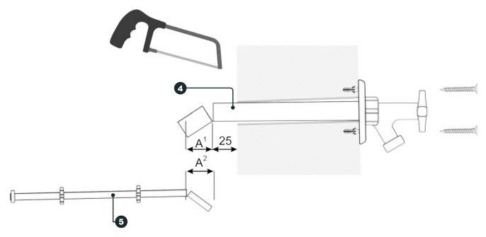
\*The length cut (A2) from the spindle (5) must be exactly the same as the length (A1) cut from the copper pipe (4).
