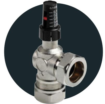
A sudden pressure increase activates the differential pressure control valve, to prevent an excessive drop in the water circulation in the central heating system. The differential pressure control valve also prevents annoying noise and ensures a sufficient flow rate, which prevents the central heating system boiler pump from overloading.
